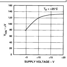
Figure 14. V<sub>IOS</sub> vs. Supply Voltage
